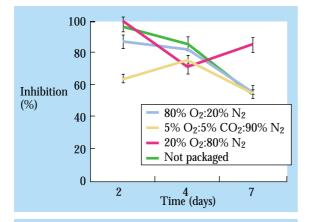
**Figure 5** The effect of packaging gas on strawberry antioxidant status. Both packaged and non-packaged fruit were stored at 8°C
