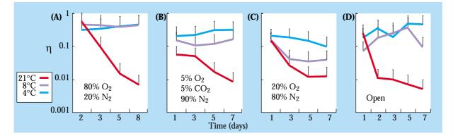
**Figure 4** The effect of packaging gas on cellulase activity. NB. Cellulase activity is inversely proportional to viscosity in this assay.
